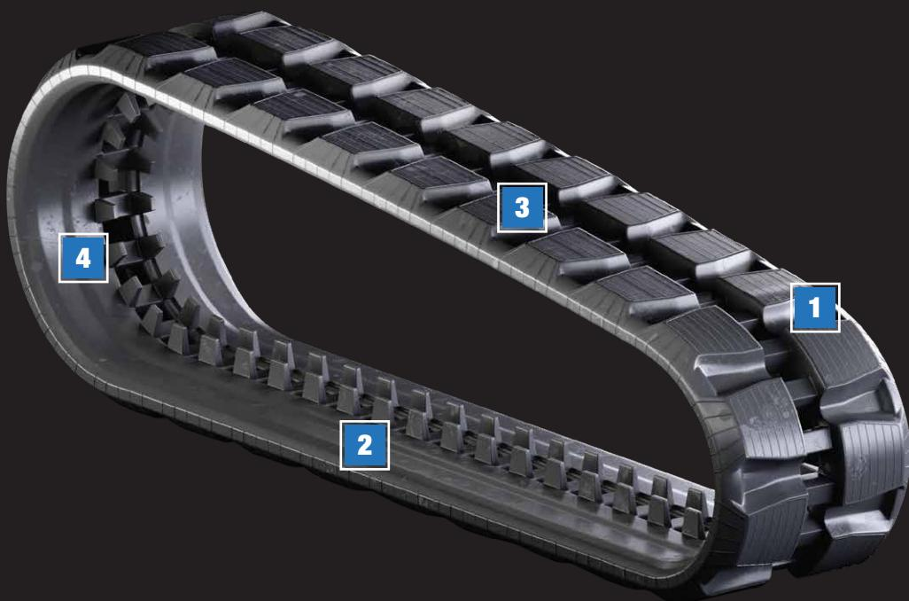
**1** Redesigned the tread pattern by adding the Hercules Armour between the treads to absorb machine operating forces and protect the track from the outside. Resulting in a massive 16.5% decrease in stress on the track.
